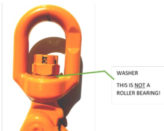
Typical swivel found on the end of a chain sling
