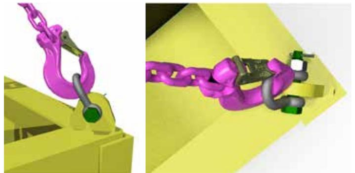
**Alignment problem - The lug seems aligned to the sling, but isn't. if the chain is short or poorly rigged it may have a pronounced twist.**
