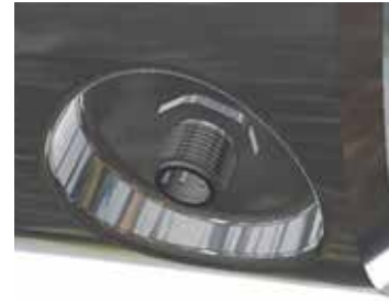
Connector in underside of Load Cell head
